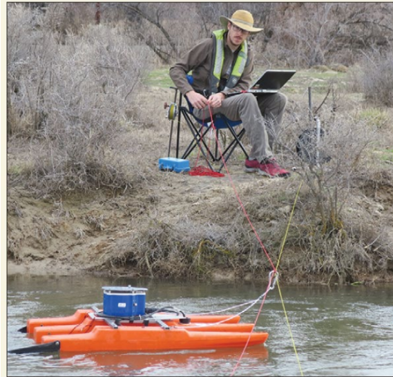
U.S. Geological Survey hydrographer making a stream-discharge measurement in Sand Run Gulch near Parma, Idaho. Photograph by James R. Bartolino, March 14, 2017.
